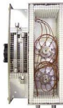
Dual TO-14 Concentrator (four traps, two valves)
