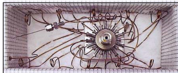
22-port stream selector valve on our 10 position Method 5030 Purge & Trap Autosampler
